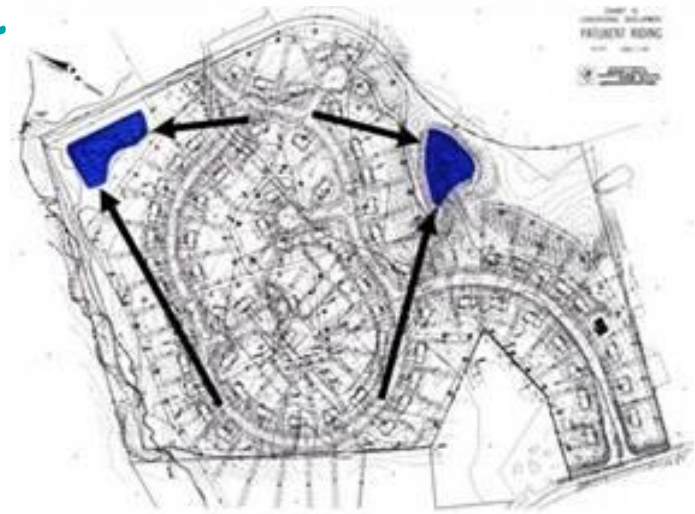
Conventional “end-of-pipe” approach
